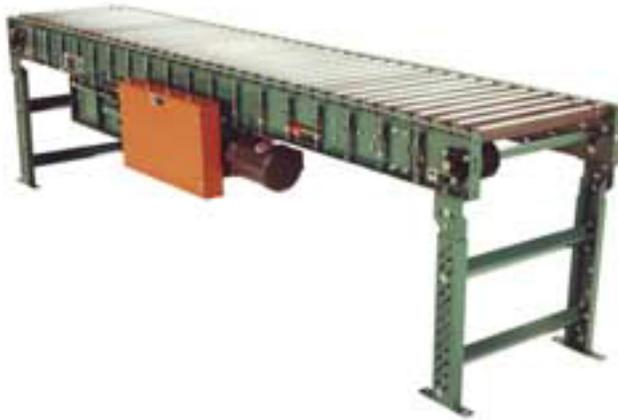
138VP accumulates goods safely and with minimum back pressure. Reversible, it can transport loads up to 100 lbs./ft. with as little as 2-1/2% back pressure. Ideally, packages of uniform weight can be accumulated temporarily using pneumatic package stops.
