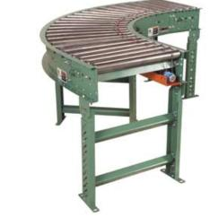
Model 738LSC features tapered rollers to help product maintain orientation. NO drive is required since it is designed to be driven from 738LS straight line shaft driven sections and includes close roller centers as a standard feature.
