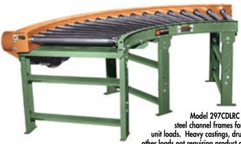
Model 297CDLRC features structural steel channel frames for conveying heavy unit loads. Heavy castings, drums and numerous other loads not requiring product orientation may be transported on this heavy duty chain driven live roller curve.
