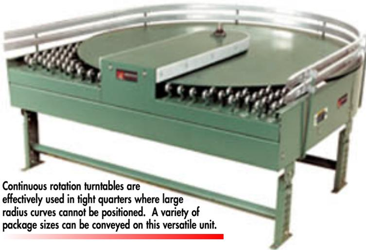
Continuous rotation turntables are effectively used in tight quarters where large radius curves cannot be positioned. A variety of package sizes can be conveyed on this versatile unit.
