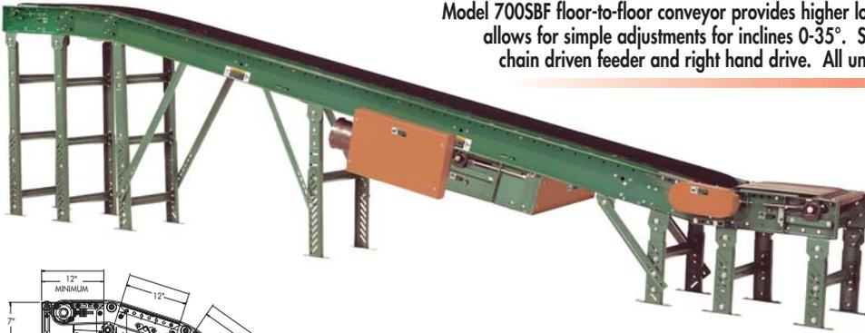
Model 700SBF floor-to-floor conveyor provides higher load capacity, reversible flow and nose-over allows for simple adjustments for inclines 0-35°. Shown with optional supports, knee braces, chain driven feeder and right hand drive. All units furnished standard with left hand drive.
