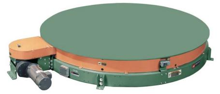
Indexing powered turntables convey heavy unit loads in numerous applications. A heavy duty chain driven live roller may be mounted on turntable platform and rotated to orient product at specified intervals allowing operator to perform a variety of tasks.
