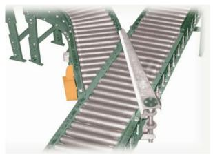
Pneumatic diverters are used to divert packages off main conveyor line onto spurs. This diverter may be utilized in powered or gravity conveyor applications. Conveyors shown are optional.
