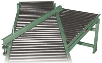
Manual diverters are used to divert packages off of a main conveying line onto other conveyors. Diverter can be used on powered or gravity conveyors. Conveyors shown are optional.
